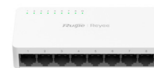
RG-ES08G-L 8-port 10/100/1000 Mbps unmanaged non-PoE switch
