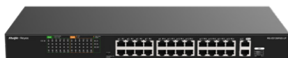
RG-ES126FGS-LP Unmanaged PoE switch with 24 x 10/100BASE-T ports and 2 x Gigabit ports
