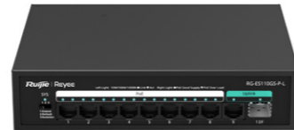
RG-ES110GS-P-L 10-port 10/100/1000 Mbps unmanaged PoE switch
