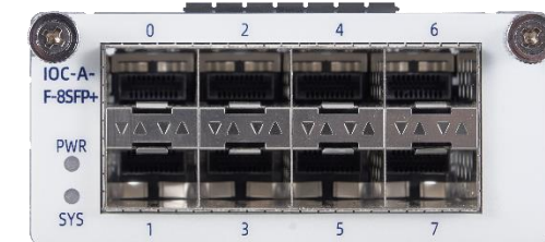
8SFP+ expansion module for front panel
